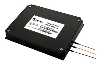
GouMax's UMI optical interleaver is a 3-port passive fiber-optic device that is used to separate Dense Wavelength-Division Multiplexing (DWDM) channels into two groups of signal streams (odd and even channels) in an interleaving way. GouMax's UMI optical interleaver uses an innovative design that features wide stopband and higher channel isolation. It provides the best solution to expand wavelength channel counts in DWDM system.
